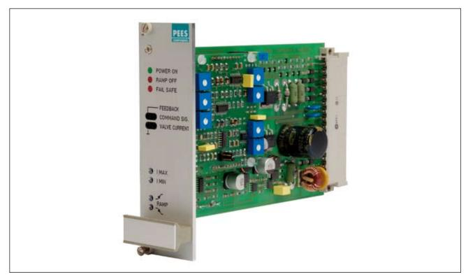
The AN533 servo amplifier has been designed to control single-magnet proportional valves and throttle valves with position controller.
