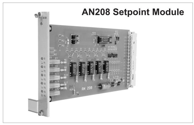
The AN208 setpoint module was designed for the application of setpoints in electrohydraulic open and closed loop control systems. With this module, it is possible to connect external setpoint potentiometers or the setpoints that are adjustable on the module can be connected internally. If external setpoint potentiometers are used, the internal multi-turn resistors can be used to extend their setting range.
