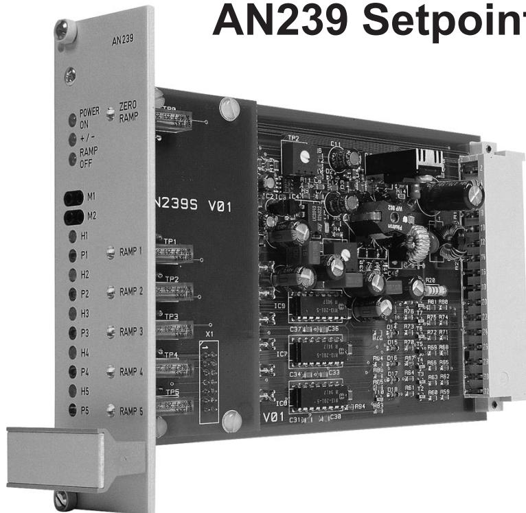
**The AN239 setpoint module permits universal setpoint switching in electro-hydraulic open and closed loop control systems.**
